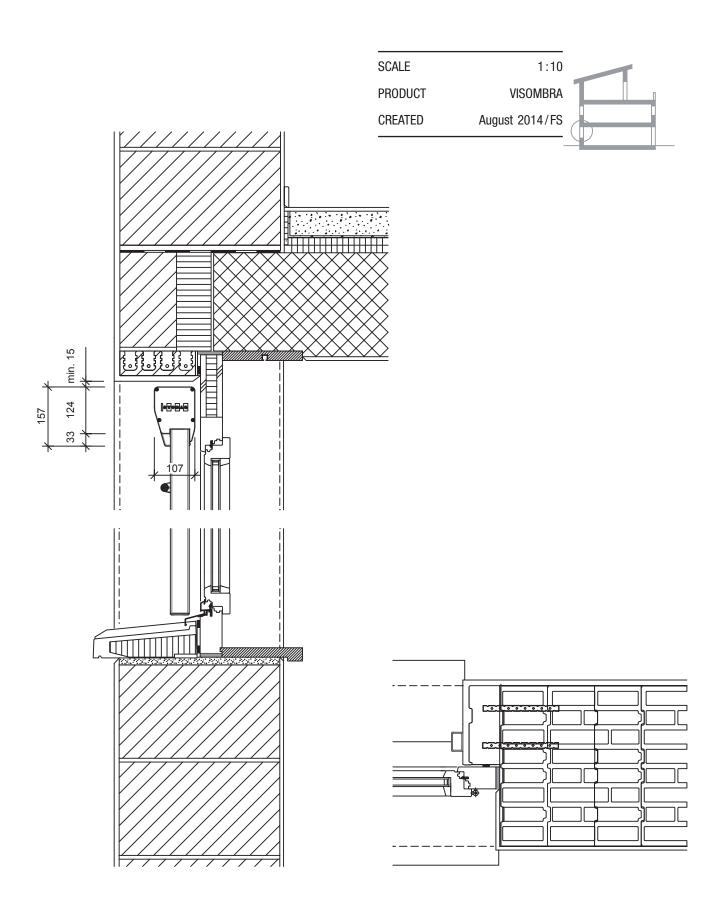
Folding awning with wind protection and fall out area, reveal assembly
