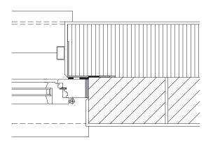
Folding awning with wind protection and fall out area, reveal assembly
