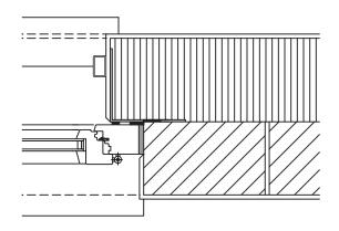
Folding awning with wind protection and fall out area, reveal assembly
