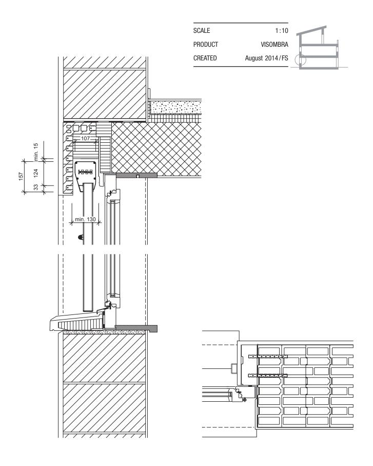
Folding awning with wind protection and fall out area, reveal assembly
